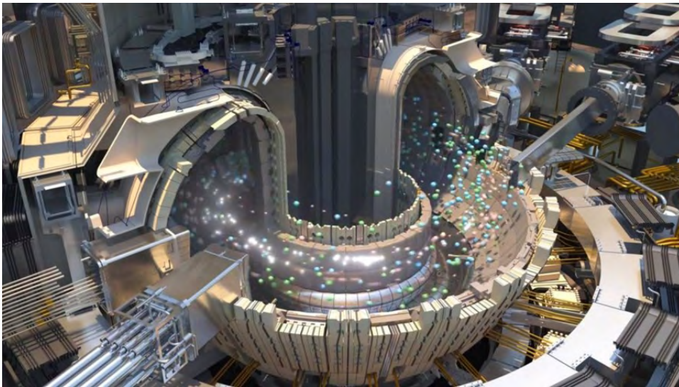
Figure 3. Tokamak Confines Plasma Using Magnetic Fields
